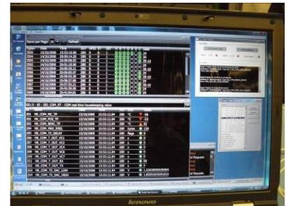
See the little window on top with all green dots? These green dots are acknowledgements that telecommands were received correctly. This picture was taken a few minutes after the first communication with the satellite entirely at  $-55^{\circ}\text{C}$ ...
