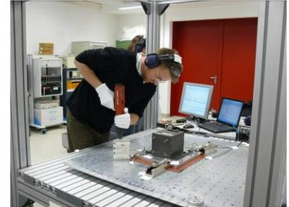
**SwissCube in the same black box is receiving gun shots (pyroshocks) to ensure it will survive the shocks created by the separation of the different stages of the launch vehicle.**
