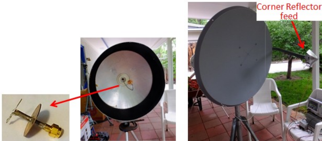
Figure 1. Center: small parabolic dish antenna (0.36m dia), Left: feed for small dish, Right: Large offset feed parabolic dish antenna (0.68m X 0.84m) showing final corner reflector feed and support arm.
