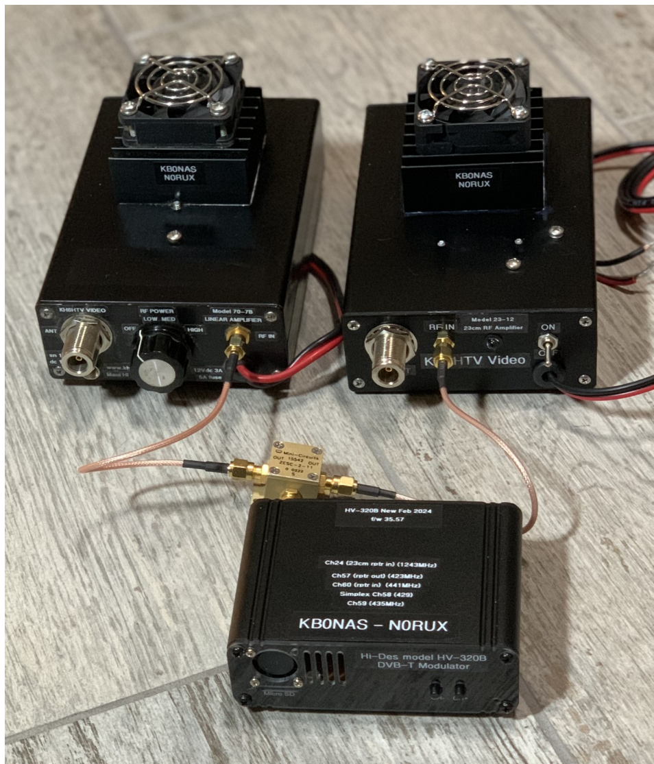
70-7B Amplifier (left), 23-12A Amplifier (right) & HV-320B modulator (front)
