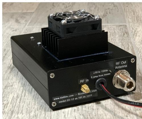
The KH6HTV-VIDEO Model 23-12, RF Power Amplifier is for use in the amateur radio 23 cm band. It is a Class A-B amplifier designed for linear service. It can be used to produce an 8 Watt (pep), analog TV or SSB signal. It can also produce a 2 Watt, high-definition (1080P), digital TV (DTV) signal. With it's low DC current draw of only 1.1 Amps at 13.8 Vdc, it is ideal for in the field battery operations, such as for ARES emergency operations.
