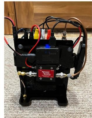
**AH2AR's new "To Go" analog, NTSC, ATV receiver and monitor**
