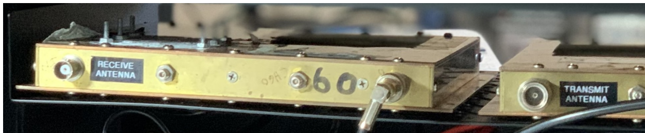
Fig. 4 Antenna Connections are found on the rear panel of the repeater.
