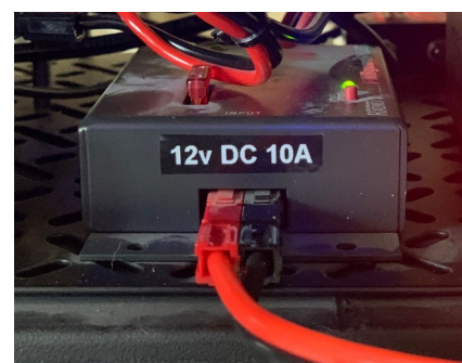
Fig. 5 DC Power Connection
