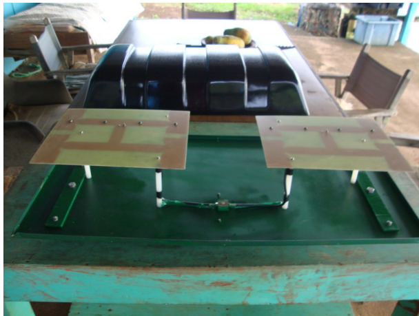
Refurbished UHF Transmitter Antenna
