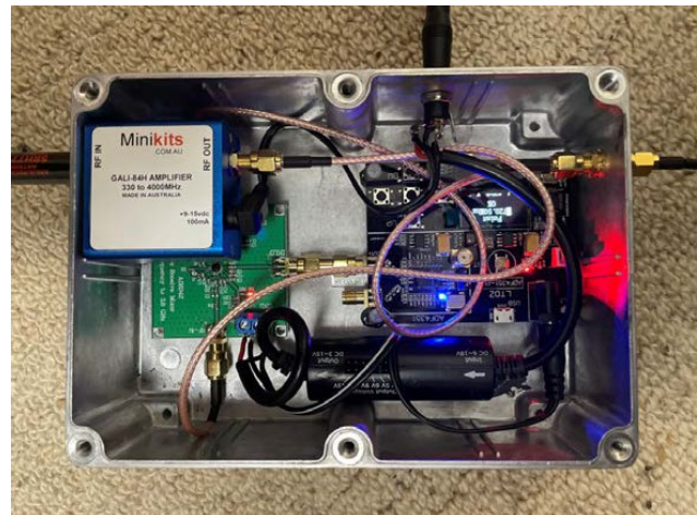
Mick's home-brew 2.4 GHz down-converter
