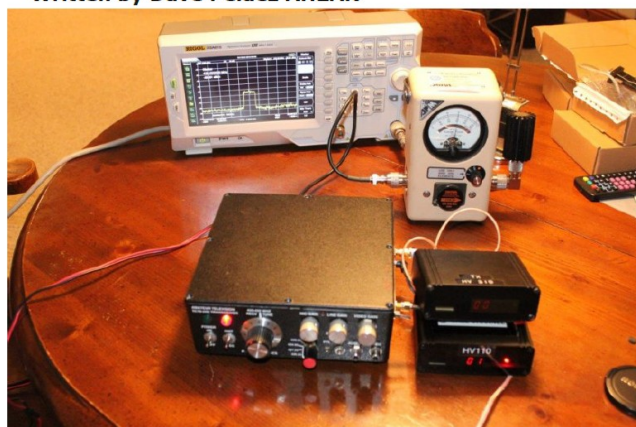
Re-purposed A5 transceiver transmitting a DVB-T ATV signal
