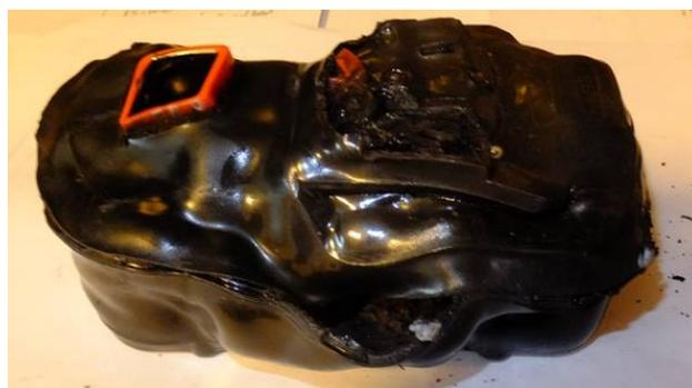
"I walked out to my garage/lab and opened the door and was engulfed in a cloud of dense black smoke. I had a meltdown of a lithium polymer battery pack for an electric drill (unknown brand Chinese import, purchased ~2 years ago). Apparently, the charge management circuit failed and charger
