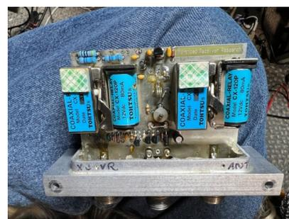
watts into the receiver section (with no RF sensing relay to switch it to pass around the active preamplifier circuit), it ended up (literally) smoking three resistors, a diode, an SMD capacitor and the MFG1302 transistor. Could it be saved?
