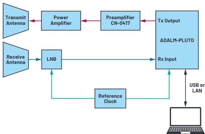
Figure 4. SDR satellite radio station.
