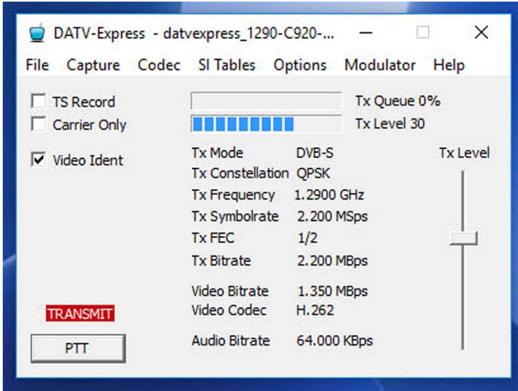
Figure 43 – The MAIN display showing normal running in TRANSMIT mode
