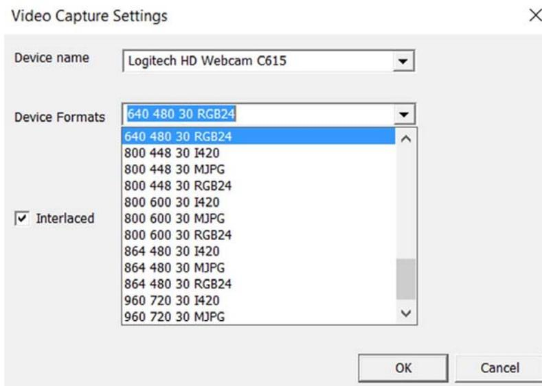
**Figure 11 – The DEVICE FORMATS menu allows a number of possible values**
