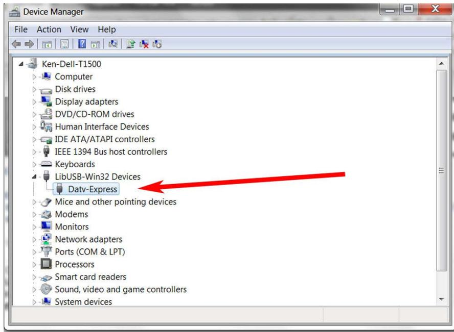
**Figure 6 – DEVICE MANAGER shows successful installation of driver.**
