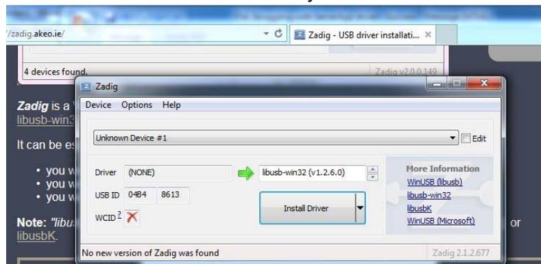
Figure 4 – ZADIG tool will install a new driver named “Unknown Device #1”
