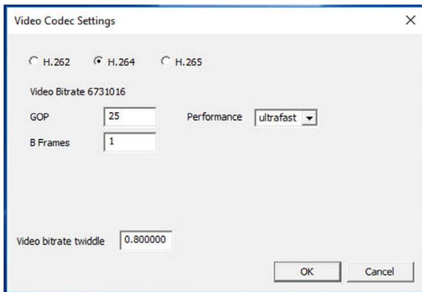
Figure 26 – Window for selecting Video Codec Settings (for H.264 and H.265)
