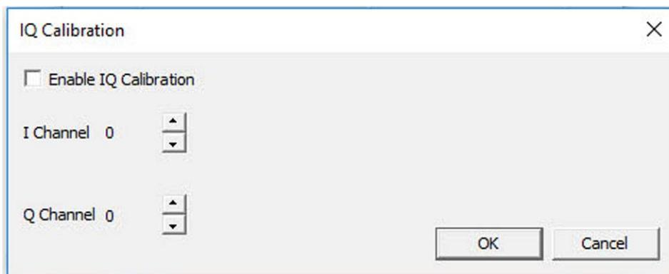
Figure 34 - Screen for adjusting DC Offset Calibration of the IQ signals
