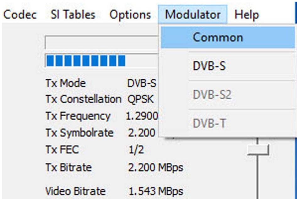
Figure 36 – MODULATOR Tab allows selecting COMMON or specific settings for three Protocols
