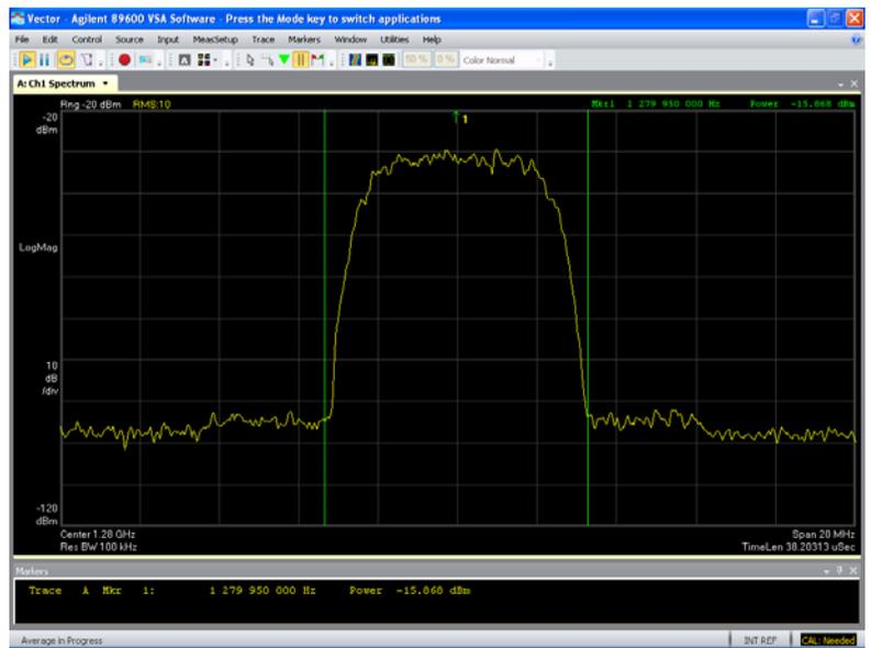
The bottom graph, taken with RF output setting = 47 (highest RF output) and external attenuator, shows higher regrowth sidebands. Regrowth is now about 10dB above the -95dB noise floor but still well within acceptable transmission limits. Here the spectral regrowth is down ~ 50dB.
