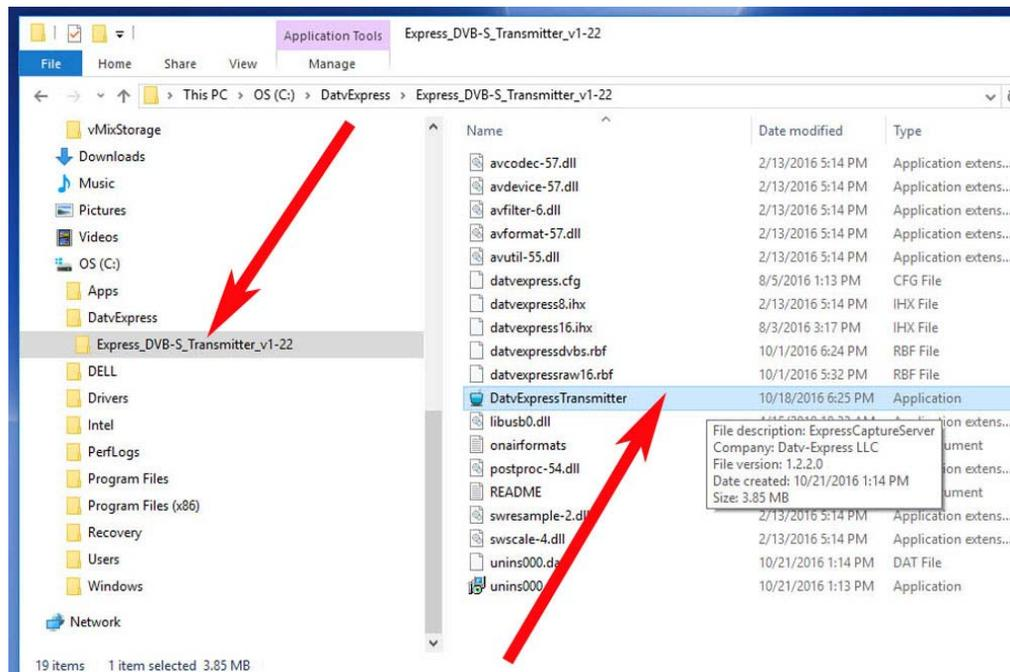
**Figure 7 – The SET-UP.exe should be allowed to default to installing software inside a Directory called DatvExpress (see left arrow)**
