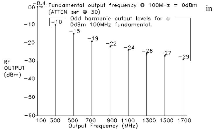
The graph at the right illustrates how the RF output decreases as the output frequency increases. At software-controlled RF output setting = 30, a 100MHz 0dBm signal reduces to about -5dBm at 1800MHz, everything else remaining the same.
