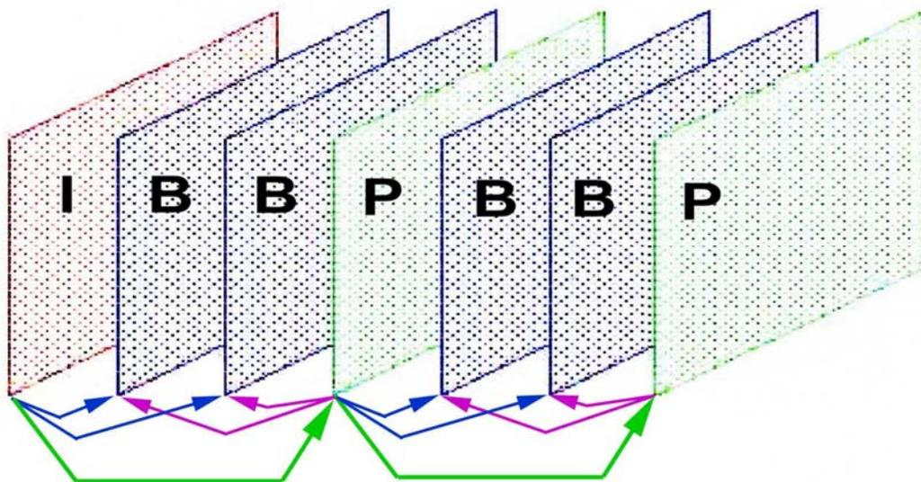
Figure 27 - A diagram of a Sequence of Compressed Frames (using the GOP mode called IBBP) that is: the B-Frames count is 2 (with GOP set to 7) (courtesy of TechTalk85)
