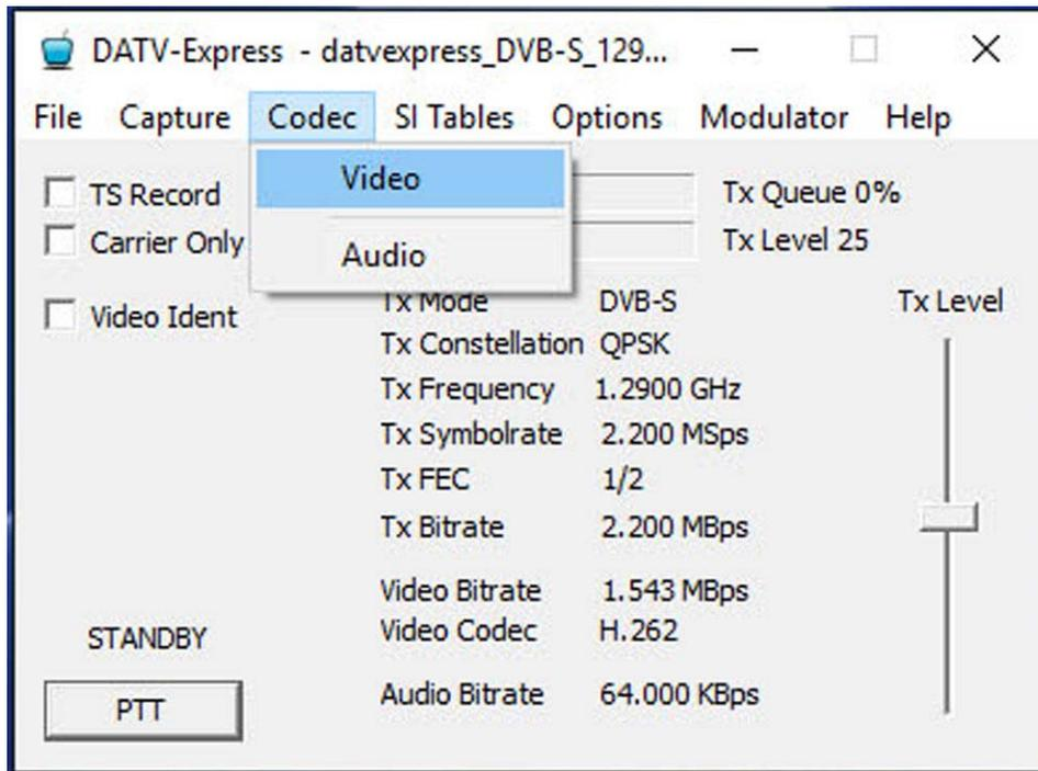
Figure 24 – Window for selecting VIDEO or Audio encoders
