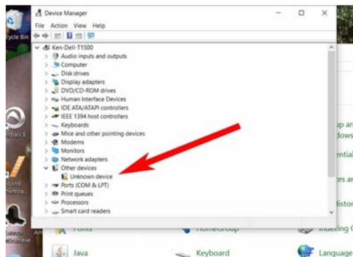
Figure 3 – Before using ZADIG, connecting Hardware Board will result in “Unknown device” driver appearing in DEVICE MANAGER
