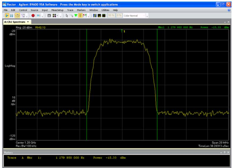
The middle graph, taken with the software controlled output = 40 and external 20dB attenuator, shows slightly visible regrowth on each side of the main signal. It raises the noise floor up about 5dB resulting in distortion being down 60dB. This is still very good.
