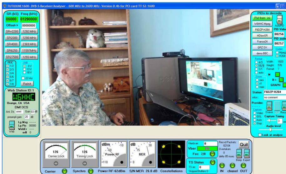
Figure 46 – Displaying H.264 video transmission in 16:9 Aspect Ratio using TuTioune Analyzer
