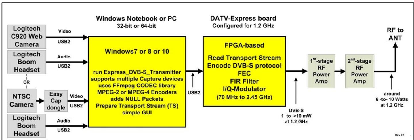
**Figure 1 – Block Diagram of typical DATV-Express board set-up with v1.23 software for DVB-S protocol**
