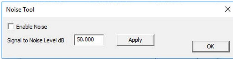
**Figure 35 – The NOISE Tool feature allows injecting noise into your Transmitted Signal**
