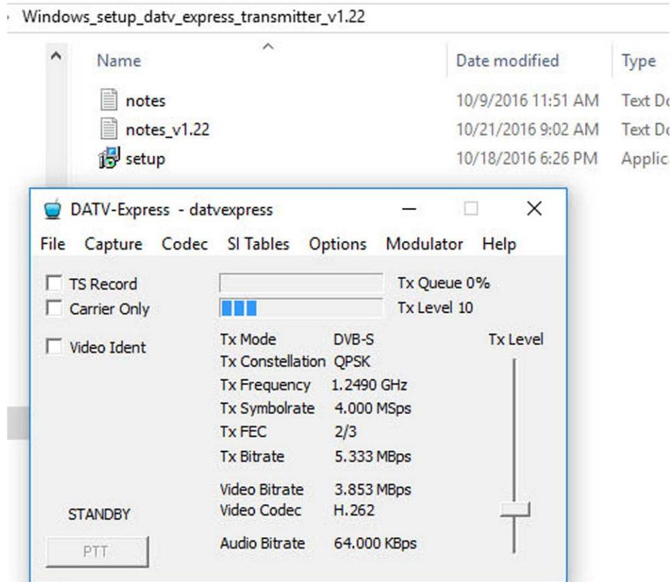
**Figure 9 – The initial MAIN screen you should see after set-up is run**
