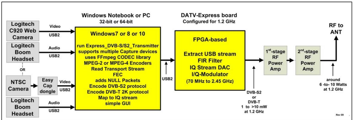
**Figure 2 – Block Diagram of typical DATV-Express board set-up with v1.23 software for DVB-S2 protocol or DVB-T protocol**
