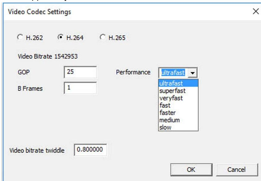
Figure 28 – Pull-Down Menu for selecting Codec Performance for H.264
