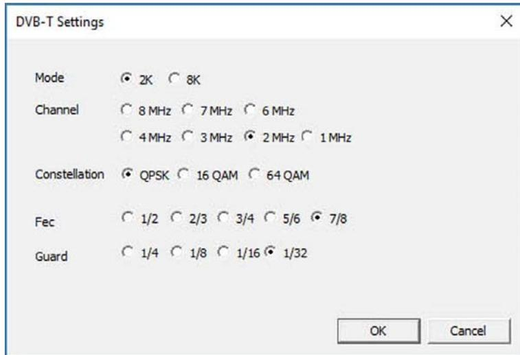
Figure 40 – Settings for the MODULATOR – DVB-T Tab
