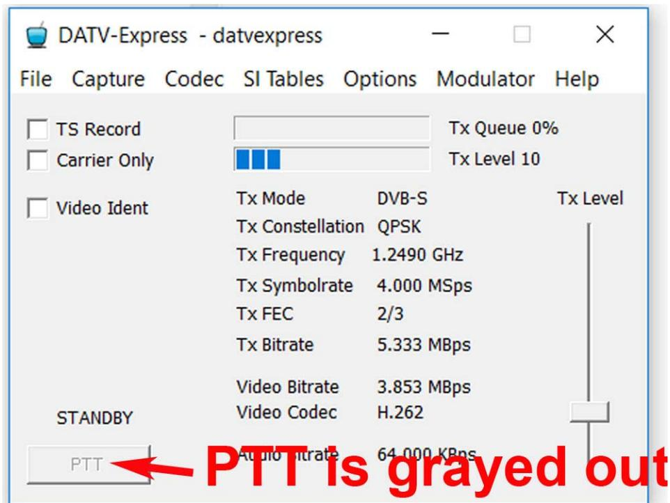
**Figure 14 – The MAIN window confirms that the software is running in the DEMO Mode with PTT button “grayed out”**
