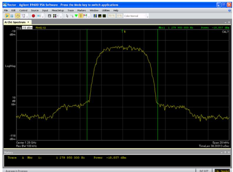
The distortion and spurs on a QPSK DATV transmitter signal should be down at least 30 dB or more from the main signal on the “after amplifier” signal. Remember when looking at the DATV-Express RF output, any post signal amplification and (or) filters will tend to add distortion and decrease the overall signal quality.
