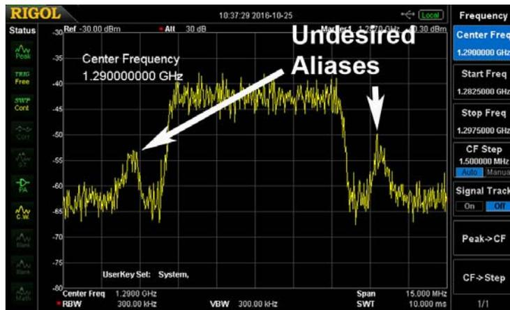
**Figure 41 – With 7 MHz Channel selected, Spikes from improperly filtered aliases appear in the spectrum when DVB-T Channel-Bandwidth not operating at 2 MHz or 1 MHz.**
