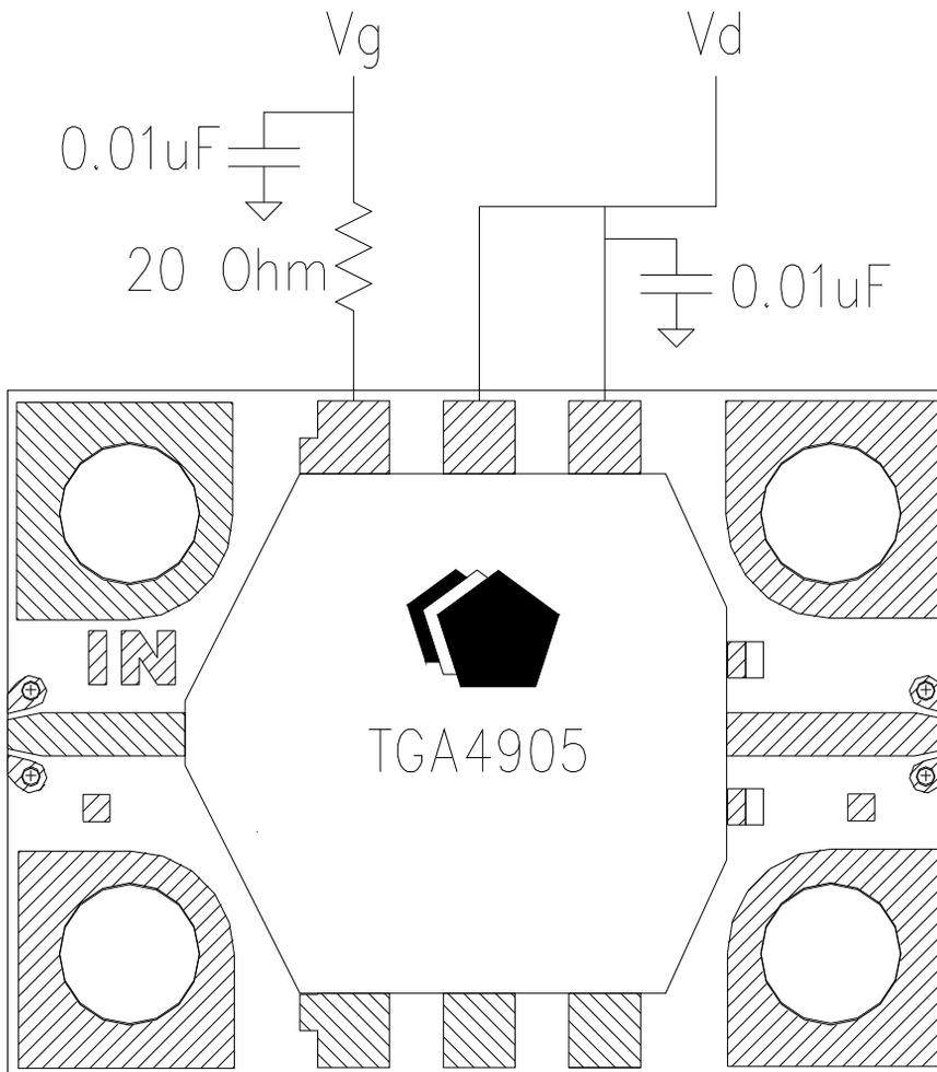
Two 1 mil wires are recommended for the RF Input, RF Output, Vg, and Vd1. Six bondwires are recommended for Vd2.
