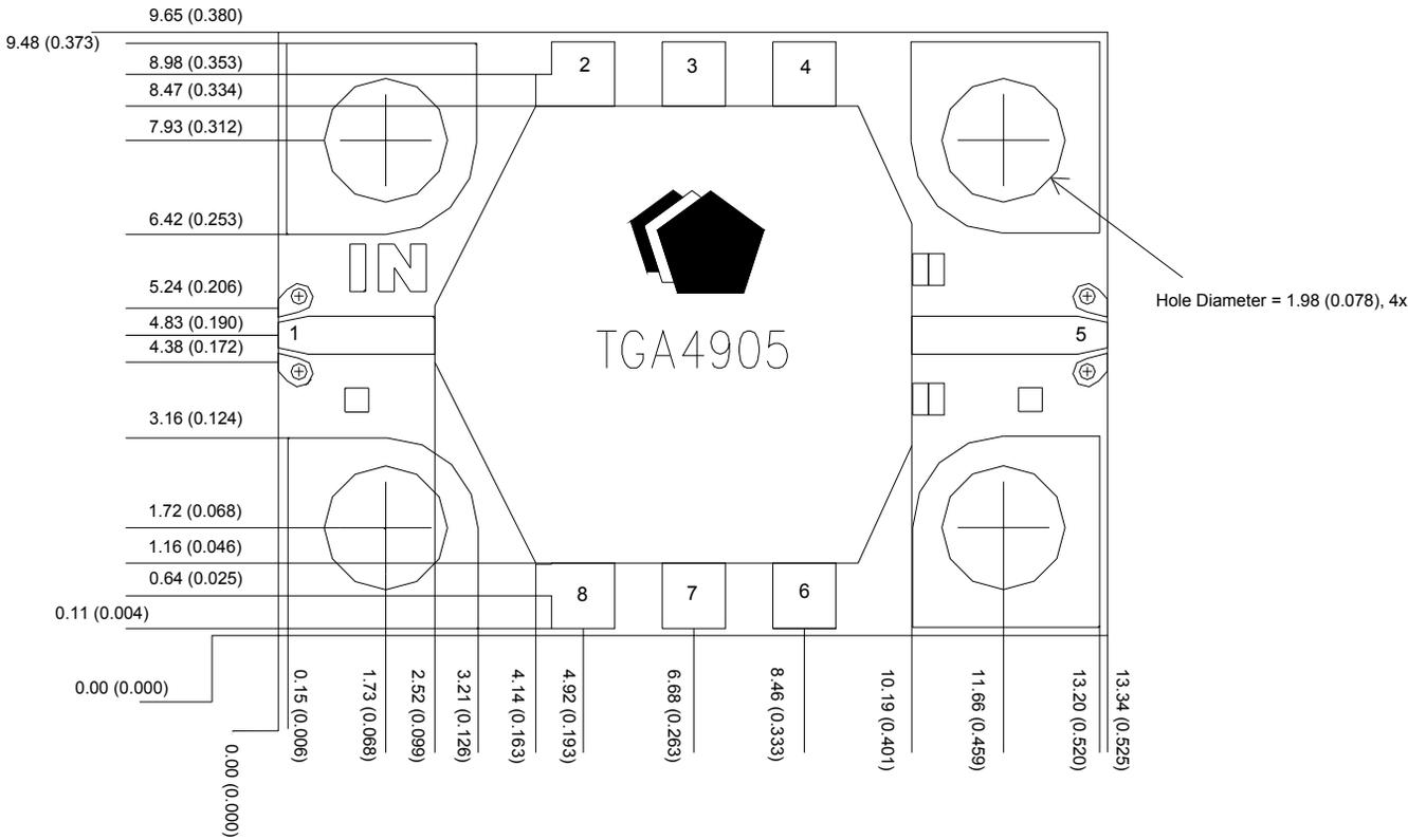
Units: millimeters (inches) Tolerance: +/-0.08 (0.003)
