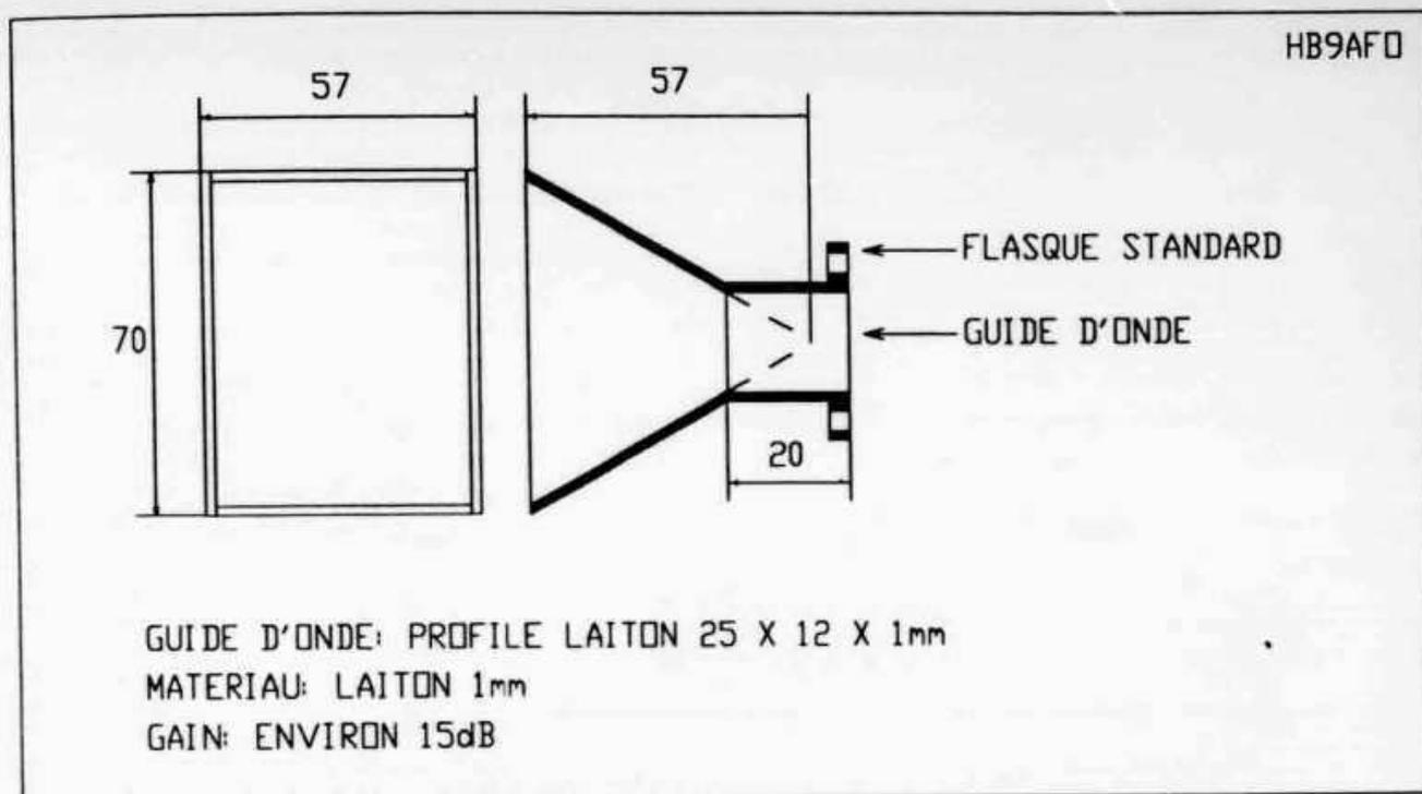
Figure 3: Antenne cornet.
