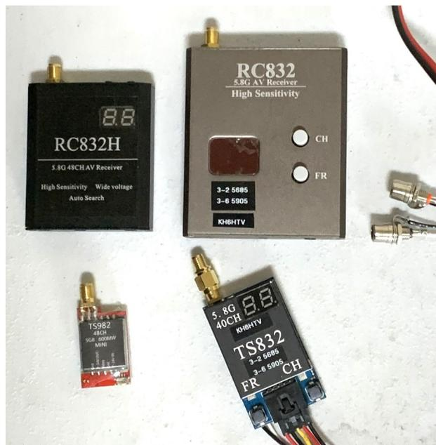
Basic RF specs. are similar, except the new units are programmed for 48 channels vs. 40 channels. But the size is dramatically smaller as shown in this comparison photo. The transmitter pc board is only 0.8" x 1.3" in size. Biggest item on it is the RP-SMA connector
