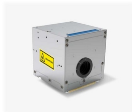
SO KD6ILO LABS © 2025 [1U FSO-2] CubeSat Optical transceiver unit for the San Diego DVB Society set for launch In late 2026 onboard SpaceX share ride program. CubeSat will be a 3U Spacecraft.
