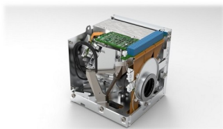
SO KD6ILO LABS © 2025 [1U FSO-2] CubeSat Optical transceiver unit for the San Diego DVB Society set for launch In late 2026 onboard SpaceX share ride program. CubeSat will be a 3U Spacecraft.
