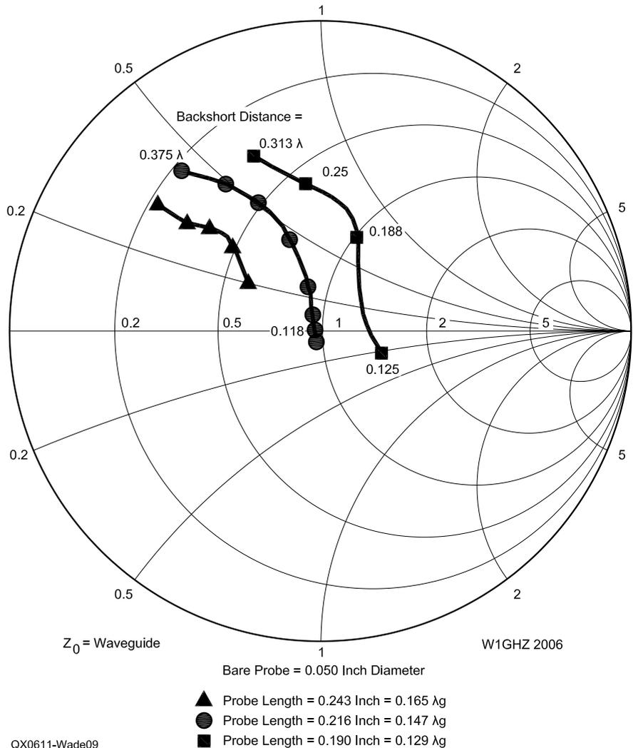
Figure 9 — Smith Chart plot of impedance as dimensions are adjusted for WR-75 to coax transition.
