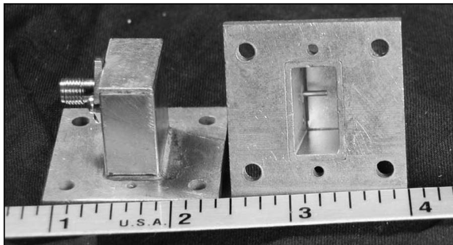
Figure 1 — WR-75 waveguide to coax transition for 10 GHz.
