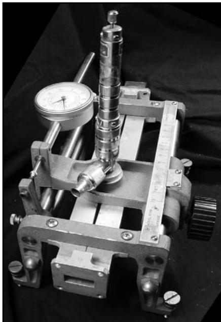
Figure 2 — A surplus waveguide slotted line.
